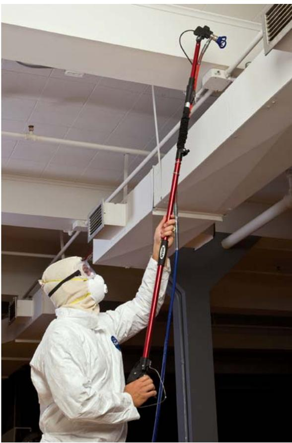
*The HYDE® RVT™ painting system lets you spray nonstop, switching easily from gun to pole as you paint. Unlike most poles, the RVT telescopes – extending your reach up to 12' with no ladders or scaffolding. You'll get faster paint jobs with less fatigue and easy clean-up.*
